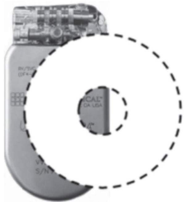
Figure 7: Placement of magnet for St. Jude or Abbott ICD 45
